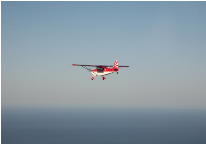
Figure 6.2 – Re-join Line – Vertical Stabiliser ½ way along the outside wing or nose ½ way along the inside wing.
