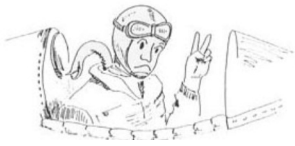
HEFOE signal followed by a number 2 would indicate an Electrical Problem
